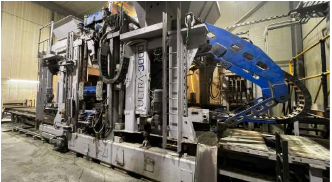
The cutting-edge Ultra-3000 is capable of producing high quality bricks, blocks and pavers at scale. Dukathole now operates nine manufacturing machines across South Africa, with a combined production capacity exceeding 90 000 tonnes per month.
