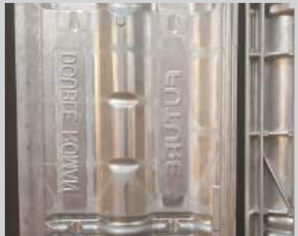
Aluminium alloy pallet cast under high pressure
