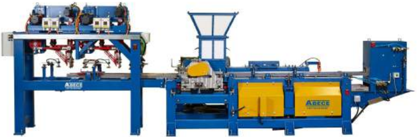
ABECE M32 extruder and double servo knife
