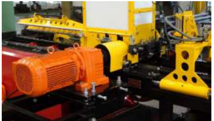
The PROTILE® P70HD, capable of extruding 100 tiles per minute.
