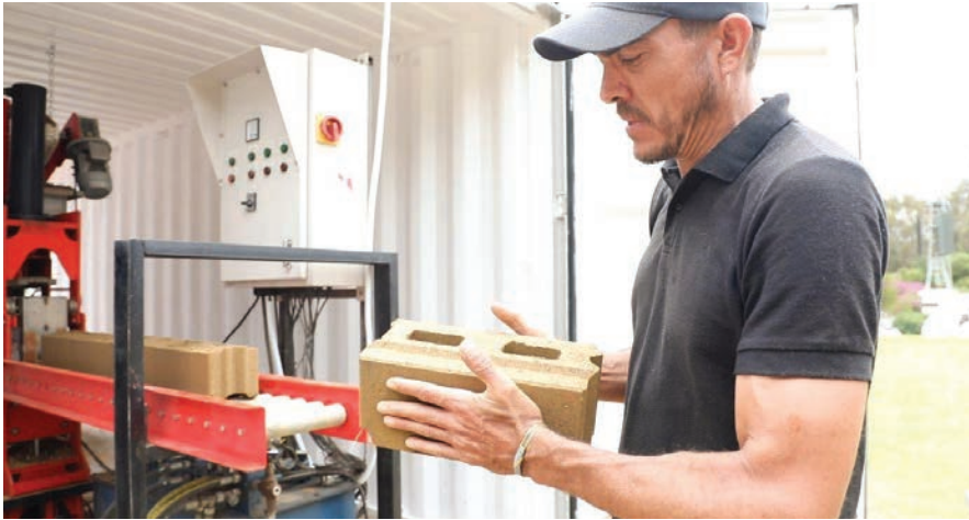
Freshly-cast Click Brick™ building blocks are conveyor-fed for easy retrieval and stacking.
