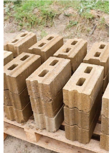
Palletised blocks are cured prior to laying.
