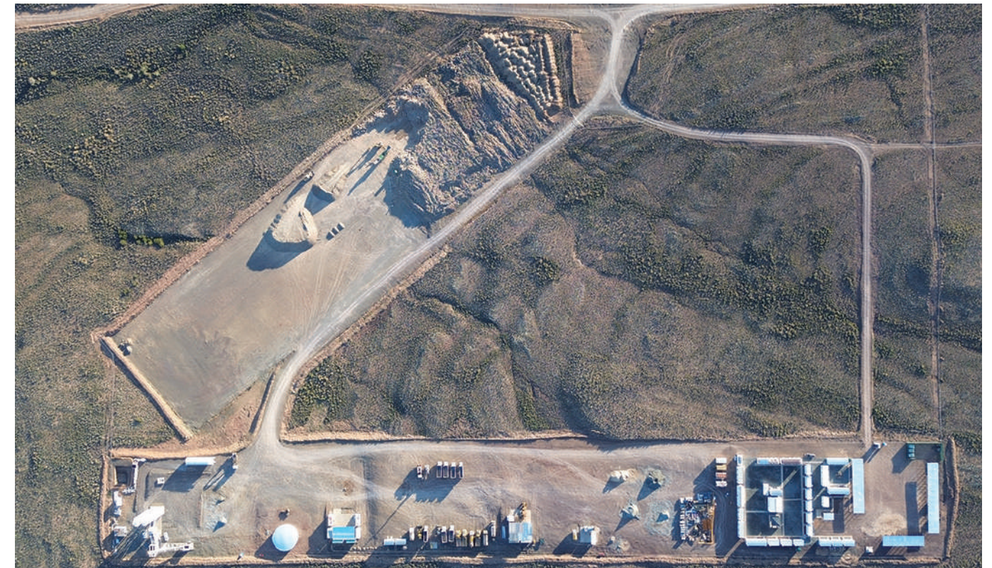
Early project works undertaken by Concor include establishing access roads, site offices and an on-site batching plant, in preparation for the large volumes of concrete needed for the turbine foundations.
