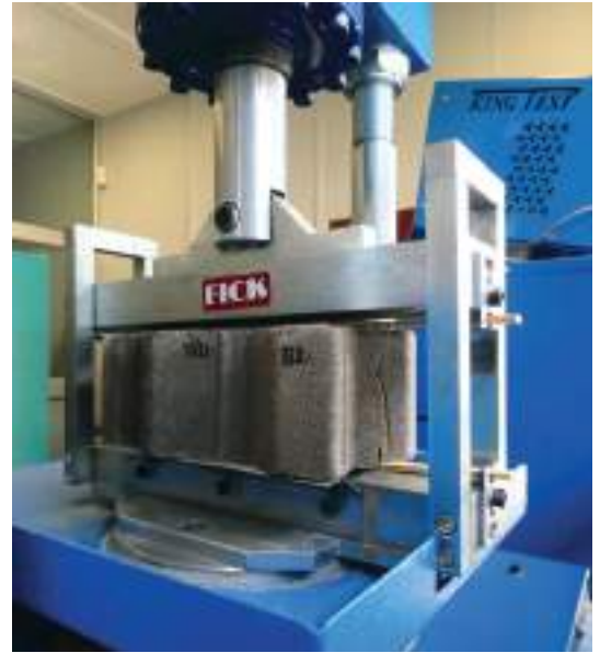
LEFT: A section of the Fick Sementwerke testing laboratory. | ABOVE: A paver undergoes the tensile splitting test.
